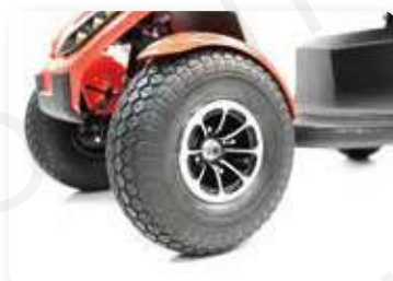
13" pneumatic tires with aluminum alloy hubs
