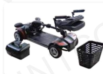
VIRGO-F Easily disassembled into four pieces
